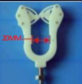
A photograph of a unilateral peach shaped wire harness fixture. Red dimensions are overlaid: the width of the opening is 20MM.                                                            |
